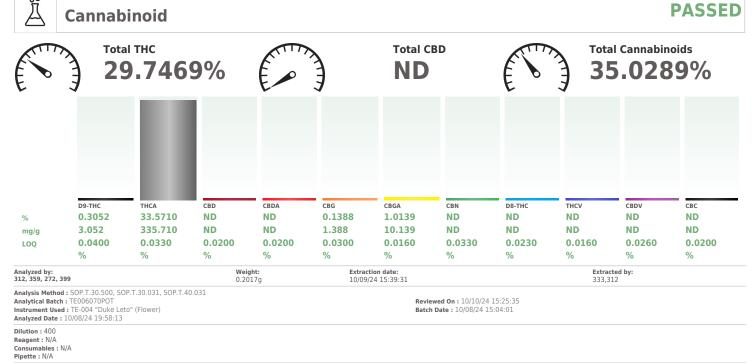
Full spectrum cannabinoid analysis utilizing High Performance Liquid Chromatography with Photo Diode Array detector (HPLC-PDA) for analysis. (Methods: SOP.T.30.500 for sample homogenization, SOP.T.30.031 for sample prep, SOP.T.40.031 for analysis on Shimadzu LC-20X0 series HPLCs). Potency results for cannabis flower products are reported on an "as received" basis, without moisture correction.
